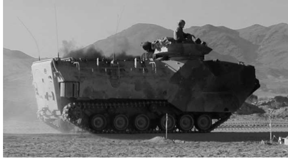
Figure 10: AAVP7A1 tracked, armored assault vehicle.
