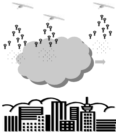
Figure 1. Tracking chemical plumes using ad hoc distributed sensors.
