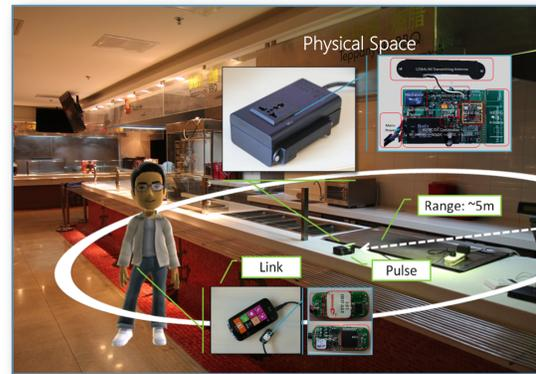
**Figure 4.** *Pulse* creates a virtual zone with magnetic beacons, which can be detected by *Link*
