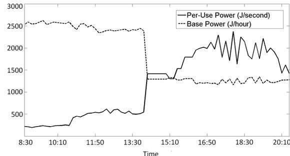
**Figure 13. The base power dominates during the day, as the fridge works to cool the interior filled with warm beverages. After that, the per-use power due to user usages dominates the fridge's energy consumption**
