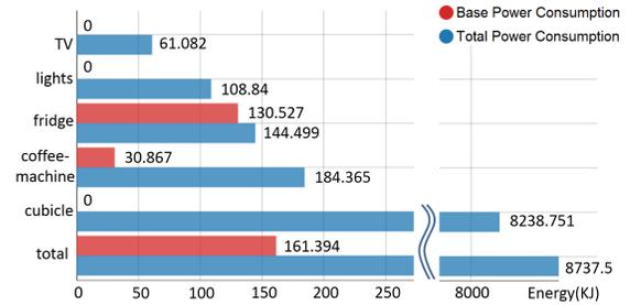
**Figure 9. User-view of total energy consumption for each device the user has interacted with**
