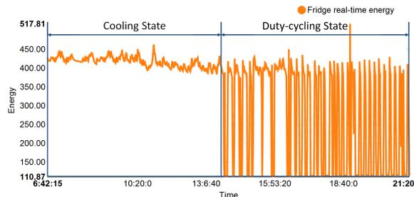
**Figure 11. Fridge energy consumption and running state**
