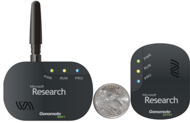
Figure 6. Two types of Genomotes designed for RAC-Net. The wireless node (on the left) controls several wired nodes (on the right) to reduce the number of wireless sensors within the same broadcast domain.
